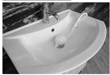
A test use has been conducted for Hand Washing with soap, with stable pressure 1,5 atm and total water consumption 3,00 lt. The clean water collection in the measurement vessel was measured 2,17 lt, water saving 72% (Manufacturer Specifications 67%).
